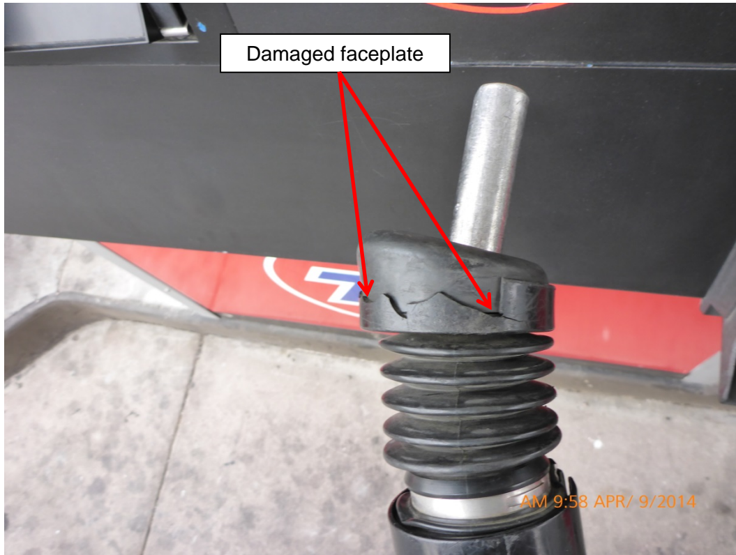
Photograph # 3: Photograph one of damaged faceplate on nozzle # 1.
