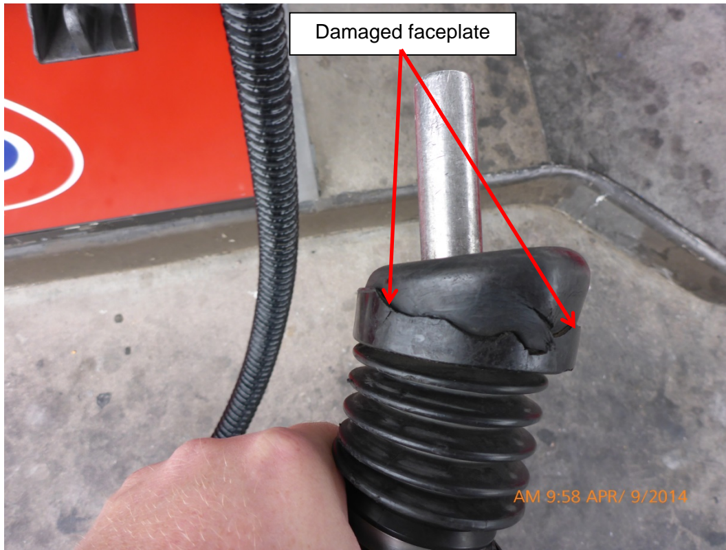
Photograph # 5: Photograph three of damaged faceplate on nozzle # 1.
